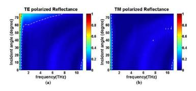
Fig. 2. Full-wave simulated reflectance spectra of the proposed structure as function of incident angles for (a) TE polarization and (b) TM polarization. The white dash curves and black dash-dot curves indicate the gradient contours for 10% and 50% reflectance, respectively.
