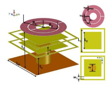
Fig. 1. A unit cell of proposed THz MM absorber.
